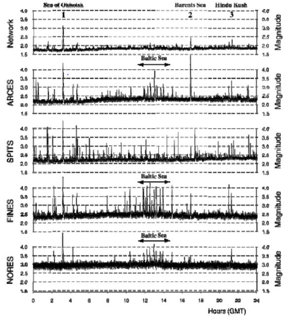
FIGURE D-4: Example of site-specific threshold ("smart network") monitoring for seismic events from Novaya Zemlya for 24 hours on February 9, 1998. SOURCE: Kværna et al., 2002
