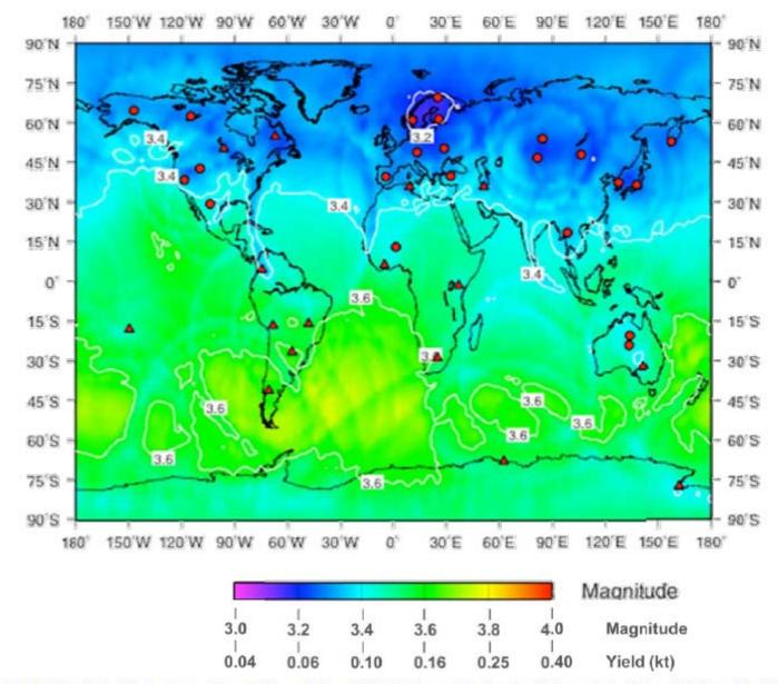
FIGURE 2-8: Detection Capability of the IMS Primary Seismic Network in late 2007, with 38 stations sending data to the IDC. Contours, indicate the magnitude of the smallest seismic event that would be detected with a 90 percent probability at three or more stations; that is, at enough stations to enable a location estimate. Red circles are seismic arrays. and triangles are 09\_25\_2012 AAAS AN-TMV.doc
